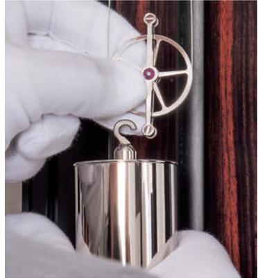
Then hang the weight in the rope pulley without bending the steel cable.
