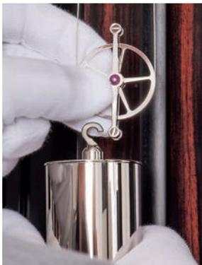
Then hang the weight in the bow of the rope pulley without bending the cable.
