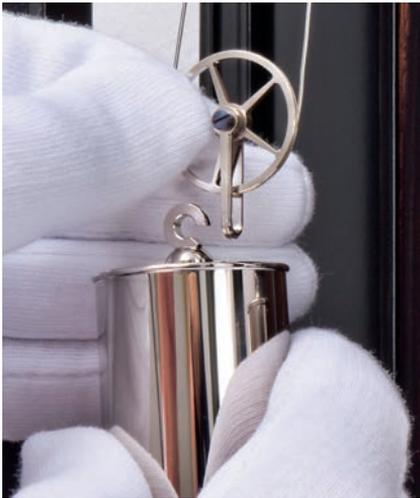
Then hang the weight in the rope pulley without bending the cat-gut.
